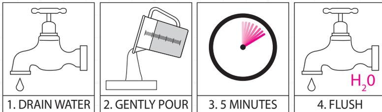
Dilute the Condensate Drain Unblocker, using 1 part product to 8 parts water, in a suitable plastic container. Once the water is added, the product will be ready to use in 5 minutes.
