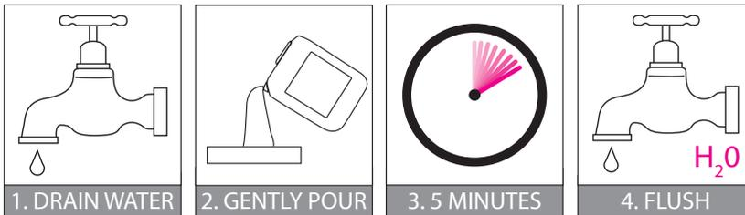
Condensate run-off from the coil will drain away slowly. If the coil is very dirty, some of this dirt will be carried into the condensate tray. Sludge and slime building up in the standing water in the tray will eventually run into the drain – causing blockages. Overflow from the tray may damage decoration and furnishings. DrainKleen® is designed for systems where a condensate pump is fitted.
