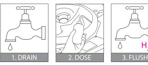
Remove excess water from condensate tray, and condensate drain, if possible. Gently pour DrainKleen<sup>®</sup> one shot into the tray and allow it to enter the drain. Allow DrainKleen® one shot to remain in the condensate tray and drain for five minutes or until obstruction is cleared. Flush out with fresh water for 2-3 minutes. Repeat as necessary until obstruction is cleared.
