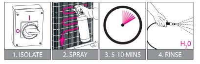
Isolate electrics. Spray into coil, starting at top corner and working methodically across and down. Rinse thoroughly with clean water after use.
