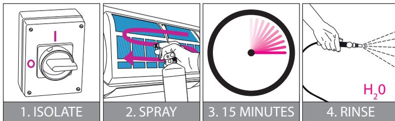
Isolate electrics. Spray into coil, starting at top corner and working methodically across and down. Keep all surfaces wet for 15 minutes. Rinse thoroughly with clean water after use.
