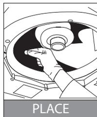
Simply place the tablet in the tray at the highest end, and adjacent to the coil, so that the resulting treatment will cover the entire tray. For larger systems multiple tablets may be used. For initial applications, or where the tray and drain are severely contaminated, double the suggested treatment rate.
