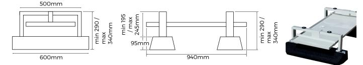
Extra clearance can be created using a **High Bloc** which fits underneath.
