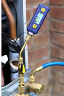
5° bend ¼ flare female connector connects directly onto the system allowing for a more accurate reading
