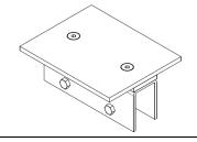
Ancillaries available include: **B9306—HD Clamp**; 2no clamps are included per HD Beam. **B5104—HD mounting plate**; available as a add-on if required.
